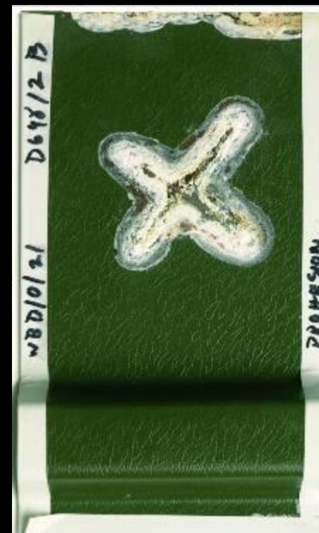
1000 hours prohesion test: ASTM G85 /
