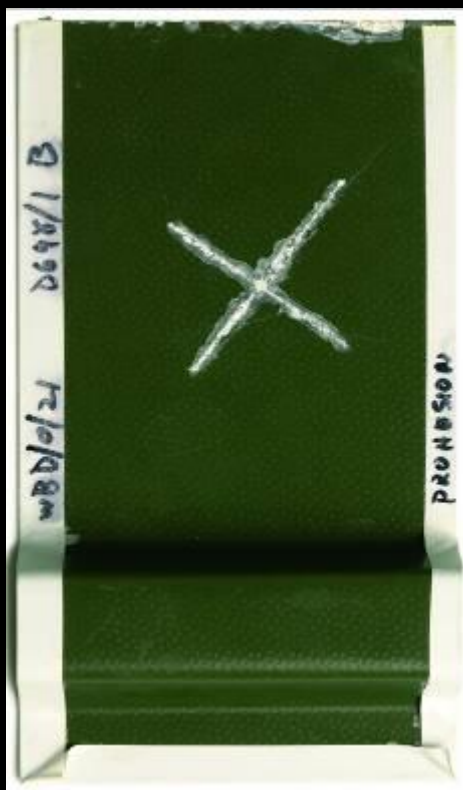
1000 hours prohesion test: ASTM G85 /
